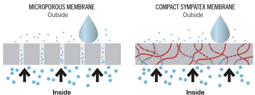
A membrane is waterproof if it can resist a pressure of
