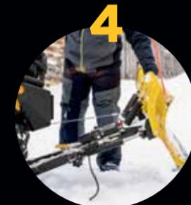
4 Remove the winch cable from the guide. You're ready to plow.
