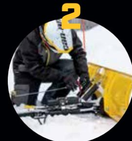
2 Attach the winch cable to the plow using a guiding hook/roller.
