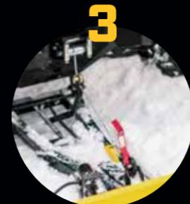
3 Lift the plow until it clips onto the mounting plate.
