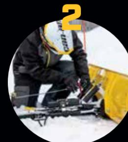
2 Attach the winch cable to the plow using a guiding hook/roller.
