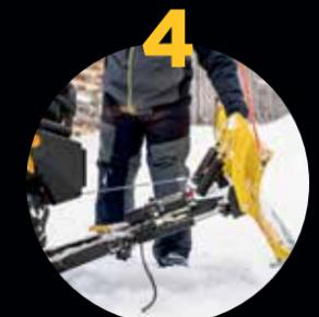
4 Remove the winch cable from the guide. You're ready to plow.
