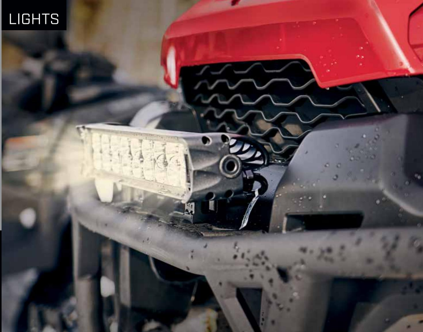
**15" (38 CM) DOUBLE STACKED LED LIGHT BAR (90 WATTS)**
